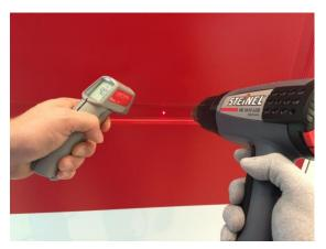
11. Remove small air bubbles first (if present), and then reheat the stretched areas up to 80-90°C. Make sure to measure the temperature of the substrate, not of the airflow!
